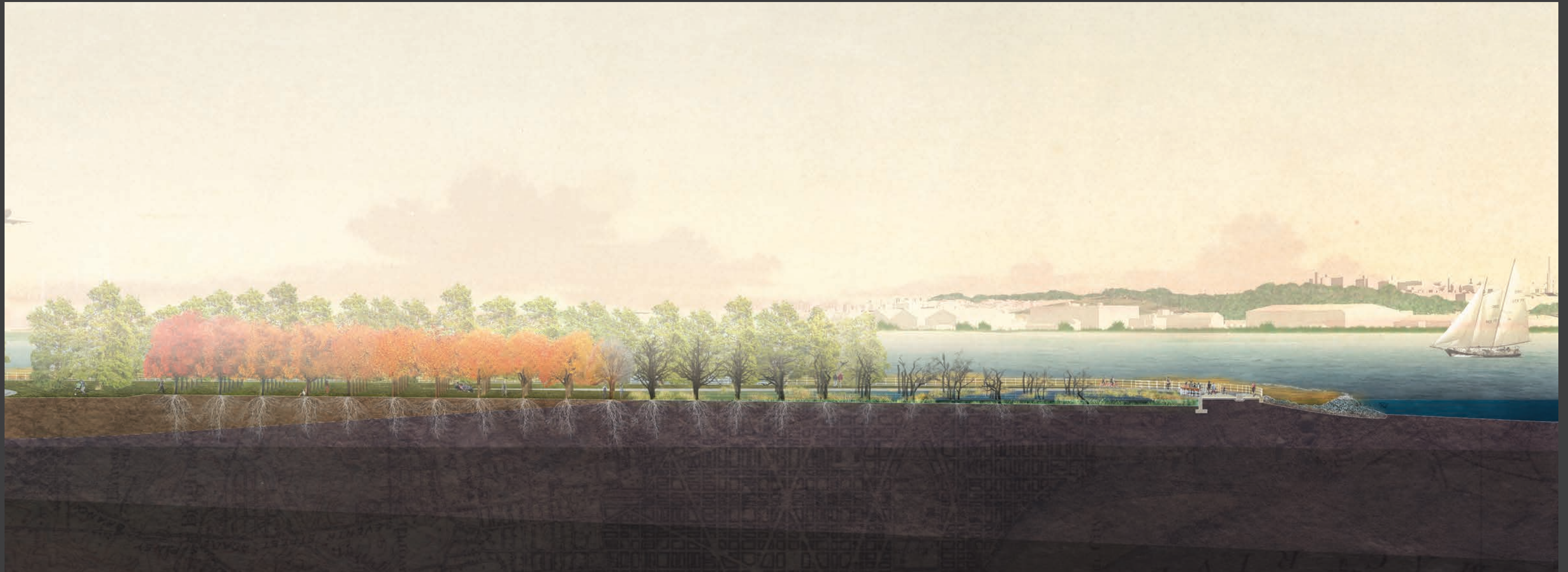
Figure 3.5 Longitudinal section of Climate Chronograph at the tip of Hains Point illustrating a gradient of inundation at a predicted future state of three feet of sea-level rise. The gradient moves from an emerging wetland at the intertidal zone through to the healthy, mature cherry trees at the highest point on the slope.
